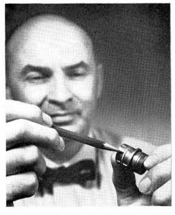
DESIGN of this beryllium copper spring band in an electrical connector earned Bob Sylvester (5512) an AEC patent. The band design minimizes the possibility of a break and eliminates the need to solder the spring in place.
